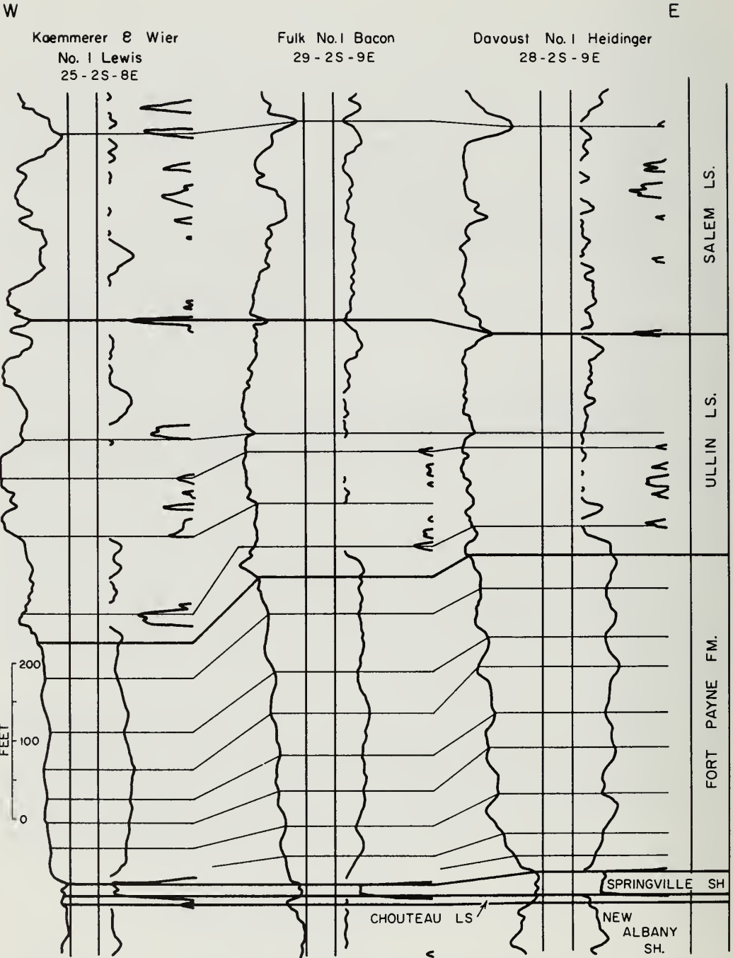
Figure 5 - Cross section showing west dip of inclined bedding in the Fort Payne Formation and Ullin Limestone on the west side of the Fort Payne tongue in Wayne County, Illinois (fig. 3).
